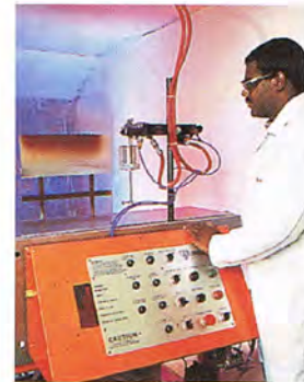
Figure 10. Comparative chip resistance test (ASTM D-3170-87) of an epoxy amine coating with KEVLAR® and with fumed silica.
